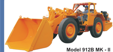
Model 912B MK - II Load Haul Dumper Bucket Capacity : 2.0 m 3
