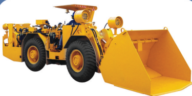
Model 811 Load Haul Dumper Bucket Capacity : 1.5 m 3
