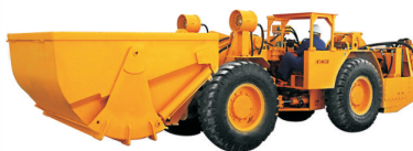
Model 912 CH Coal Hauler Bucket Capacity : 5.0 m 3
