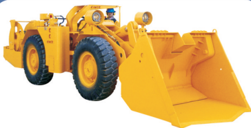
Model 912E Load Haul Dumper Bucket Capacity : up to 3.5 m 3
